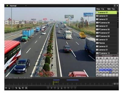
Just check the channel or channels if you want to switch playback to another channel or execute simultaneous playback of multiple channels.
